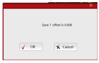
8. After saving, you can go to the "Options" column to check the safety Settings, and it will be found that the value of "work reference height" will change, because it is reset according to the value automatically tested by the machine. See below
