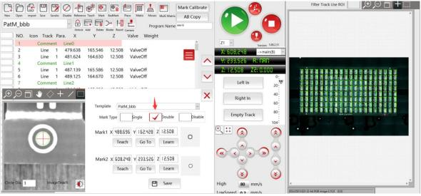
3.8.7 Move to the position of the first mark point, select main(A) main program, and place the sub-template out of the matrix in the main program, as shown below;
