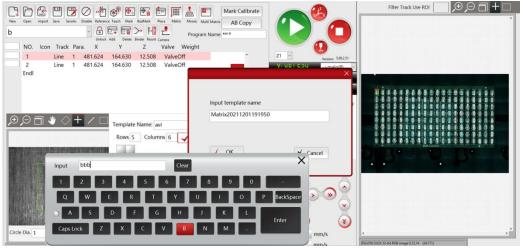
3.8.4 Input the corresponding row and column in the matrix column, and then Teach the corresponding row and column end points. The following end points of row end points are the same as the starting point set by the first board (note: to remove the check of "image teaching", you can see the cross line of the circle, that is, the center of CCD).
