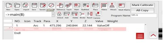
3.5 If there are many small boards with the same characteristics in a piece of board, the function of "matrix" can be used. Before using this function, a subroutine must be placed in the main program, select the placed data row, click the matrix, and operate according to the steps marked in the following picture.;
