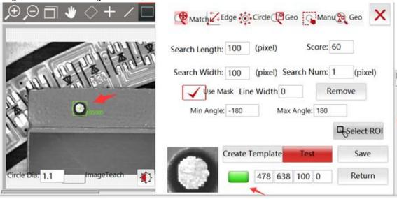
2.5 Repeat steps 2.2 to 2.4 for coordinate setting and template learning of Mark2. After setting, Click save to return to the setting interface automatically;
