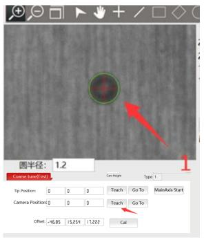
4. Finally click the "calculate" button to complete the calibration of camera and cutter head.
